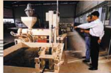
MODERN EXTRUSION LINE FOR GREASED AND POLYETHYLENE COATED UNBONDED TENDON
