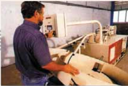
TENDON FABRICATION LINE WITH AUTOMATIC TENDON CUT OFF
